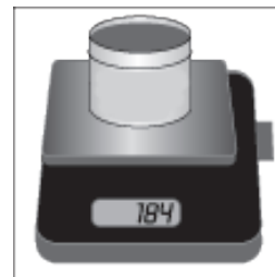
Image 4, weigh wet mass sample and can
