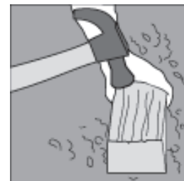
Image 2, gently tap sample can with wood block and hammer
