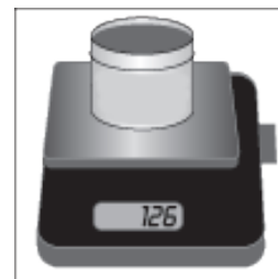
Image 6, weigh dry mass sample and can
