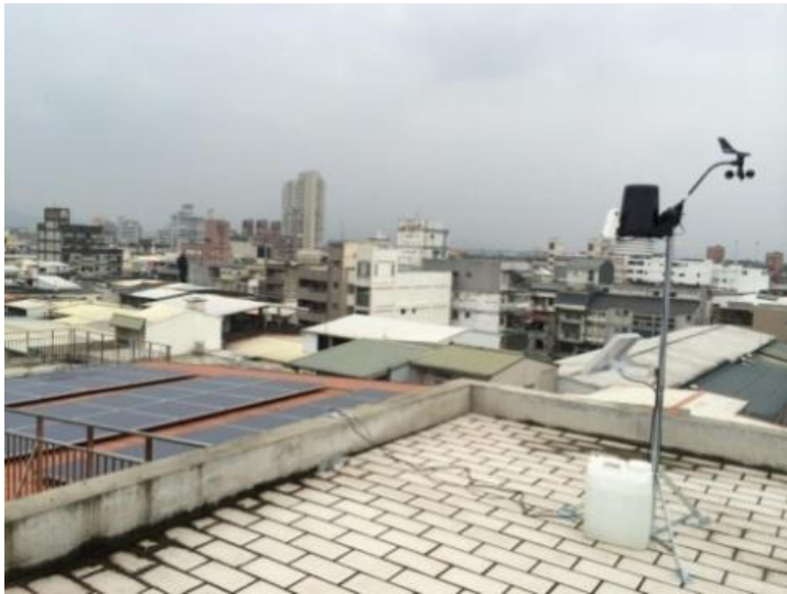
(圖 1) Davis meteorological observing system
