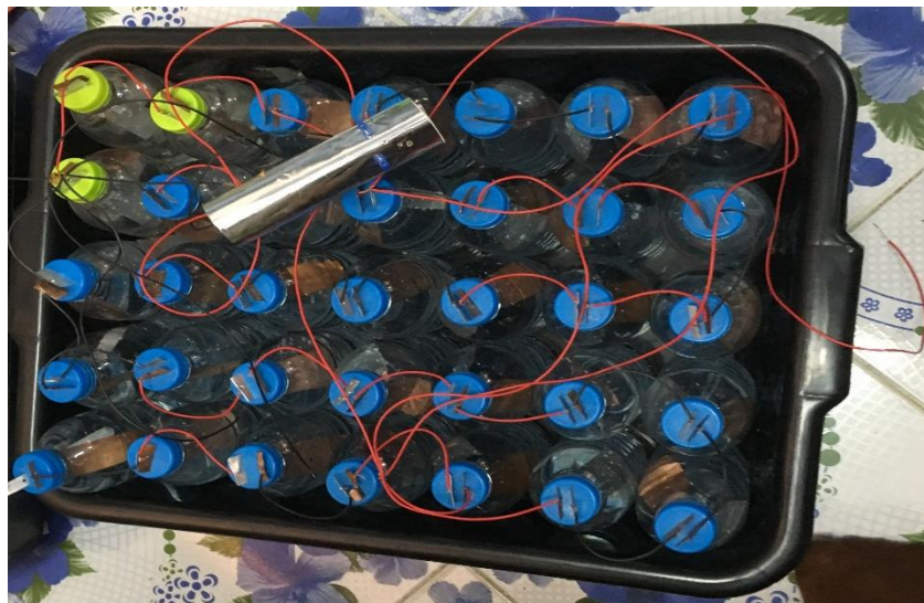
Picture 6 Connecting the battery cells
