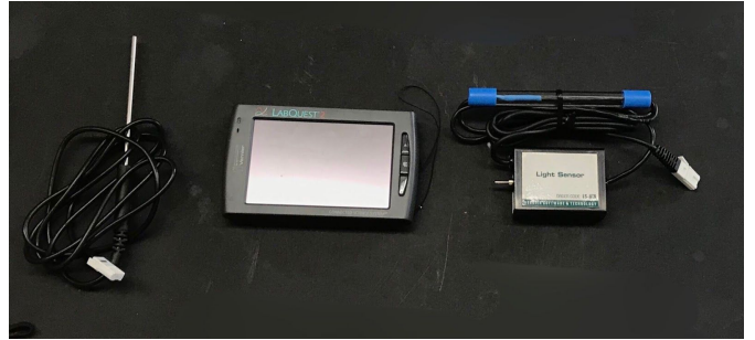
Figures 2-4: Figures 2, 3, and 4 show the devices used to take measurements the day of the solar eclipse. Figure 2 shows the chart that was used as a guide by the student researchers observing clouds. Figure 3 shows the Infrared thermometer used by those measuring surface temperature. Figure 4 shows the probes for light intensity (right) and air temperature (left), which required the use of a lab quest (center) in order to record the data.
