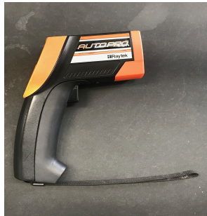
Figures 2-4: Figures 2, 3, and 4 show the devices used to take measurements the day of the solar eclipse. Figure 2 shows the chart that was used as a guide by the student researchers observing clouds. Figure 3 shows the Infrared thermometer used by those measuring surface temperature. Figure 4 shows the probes for light intensity (right) and air temperature (left), which required the use of a lab quest (center) in order to record the data.
