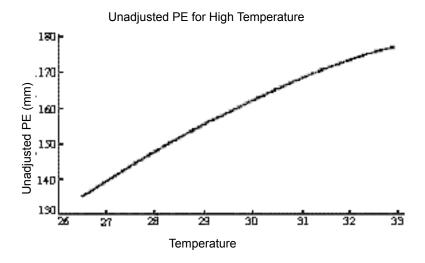
**Note:** Draw a vertical line up from temperature to the curve, then a horizontal line left from the curve to the UPE line. For example, a temperature of 27° C would have a UPE of  $\sim$  140 mm Step 5
