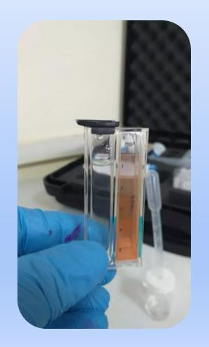
We determine iron levels using a colorimetric method.
