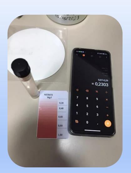
Nitrites are extremely toxic to fish and shellfish. The nitrites concentration of the sample is 0.23 mg/l.
