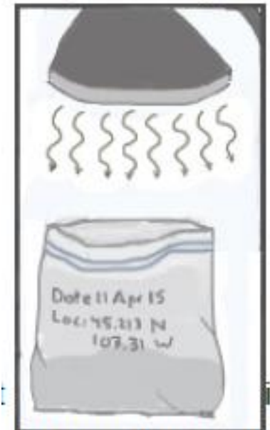
Figure 2, drying soil under heating lamp
