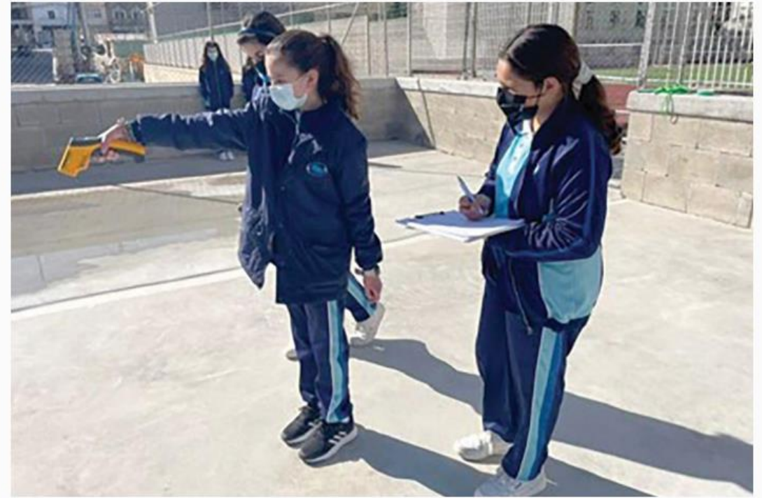
Students using an infrared thermometer to measure concrete surface temperature.
