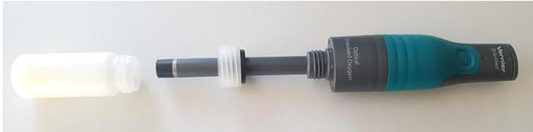
Optical probe with storage container: Insert probe into lid and carefully screw on container.
