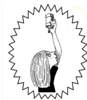
Figure 4: For the use of the densimeter the observer's arm must be fully stretched and the washer must remain perpendicular to the observer's face.
