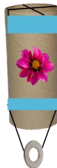
Figure 3: Densiometer made by the students. The light blue stripes are the adhesive tap strips that attach the thread to the densiometer.
