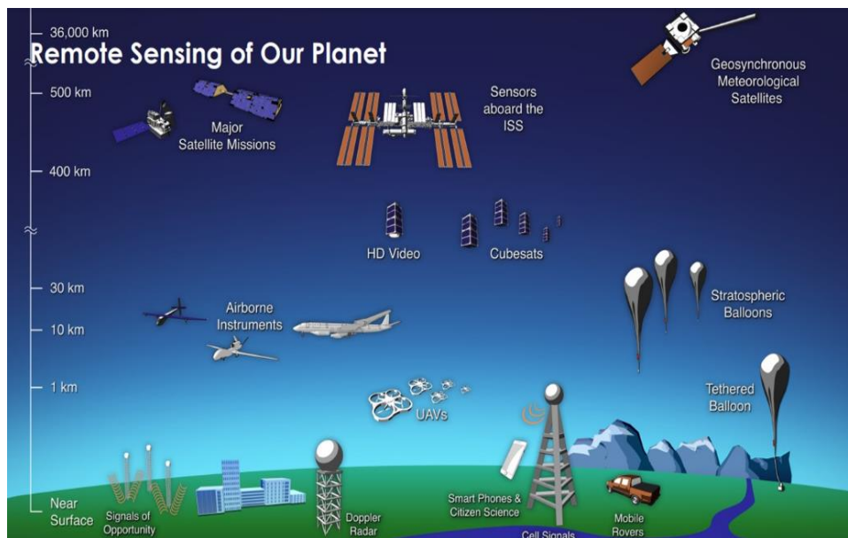
Figure. 1. Types of remote sensors that gather information from Earth. Source: https://svs.gsfc.nasa.gov/30892
