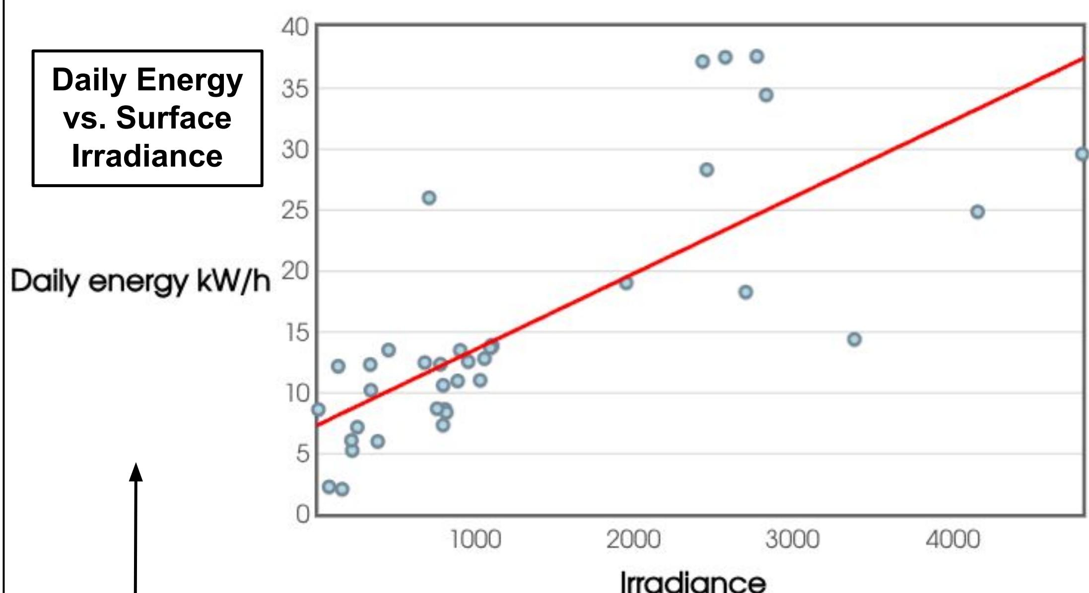
This graph displays a strong correlation between daily energy and irradiance. An increased amount of power is produced during times of high solar irradiance and it decreases during times of low irradiance.
