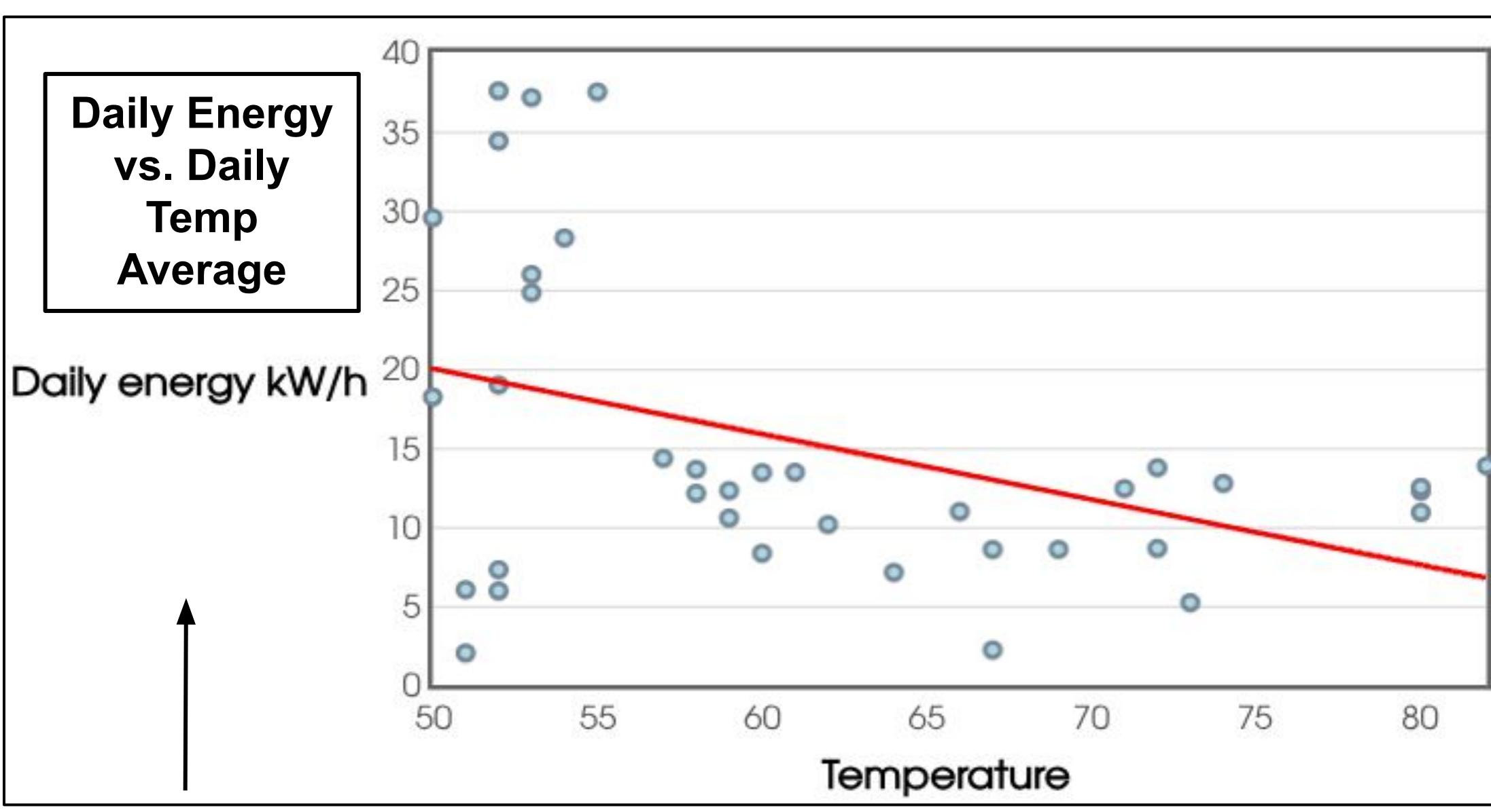
The daily energy being produced on days with higher temperatures shows a strong correlation between reduced kW production and higher temperatures. Cold weather does not mean solar panels produce less energy, often it the irradiance is significantly higher during these temperature when not disturbed by clouds.
