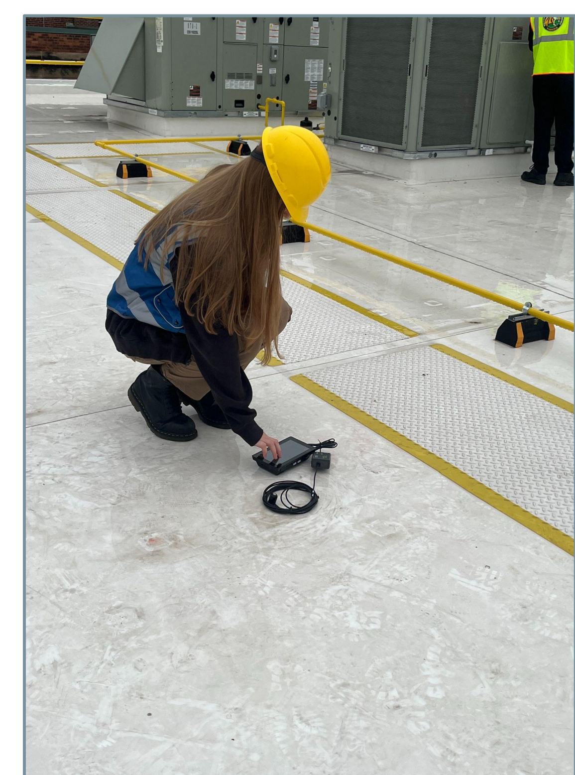
(Collecting Solar Irradiance from our buildings roof with pyranometer)
