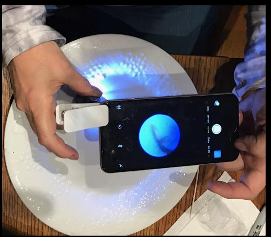
Line up the lens so that the specimen is in the circle of light on the viewer.
