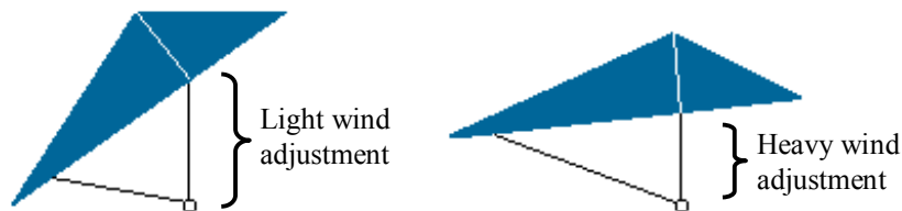
Position the bridle to compensate for the force of the wind.
