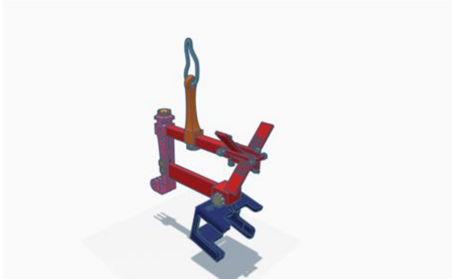
Figure 1: Redesign of an Aeropod camera mount done by students in Foundations of Engineering Lab using new and previous parts.
