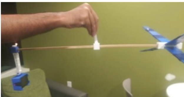
Figure 15: Redesigned Aeropod with adjustments to the tail in order to address issues with aesthetics and performance. The camera mount was also redesigned to provide for easy removal and reattachment for data collection
