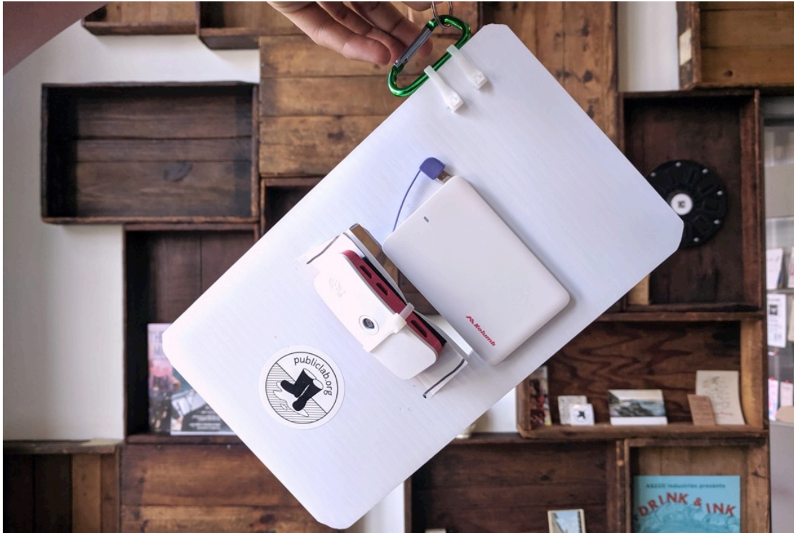
Prototype aerial rig for the Infragram Pi kit: https://publiclab.org/notes/warren/06-05-2019/build-a-simple-aerial-photo-rig-for-a-raspberry-pi-camera
