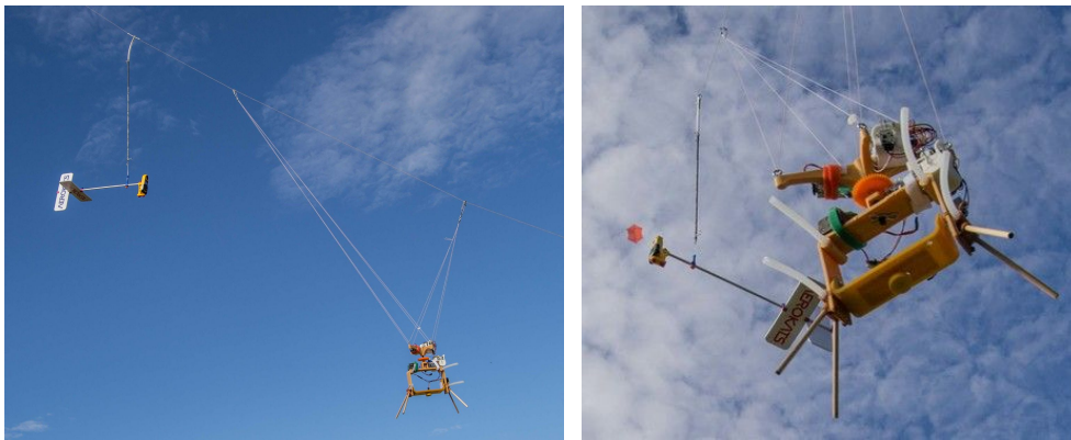
Comparison of Aeropod Prolifer with hot-wire anemometer system - see: https://publiclab.org/notes/cfastie/10-17-2017/winds-aloft-sensor-overload
