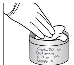
Image 10, wipe inside of sample can
