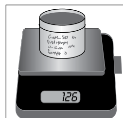
Image 8, weigh dry mass sample and can
