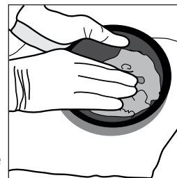
Image 12, Push dry soil through sieve
