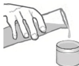
Image 11, measure volume of sample can
