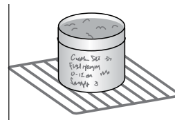
Image 7, dry sample without lid in oven
