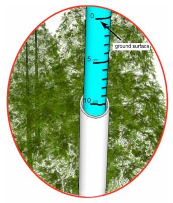
Figure 3. Ground surface and 5 cm below-ground increments with 1 cm hash marks on inner tube
