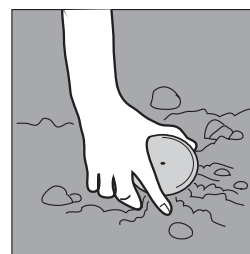
Image 1, pushing sample can into soil
