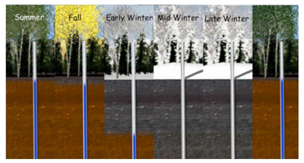
Figure 5. Progression of freezing through the seasons. Frozen ice is shown as white and unfrozen water as blue in a Frost Tube.
