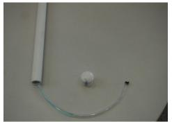
Figure 1b. Assembled Frost Tube
