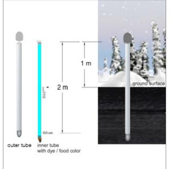
Figure 2. Frost Tube assembly showing liquid-filled inner tube (both ends sealed) and outer tube as well as the assembled frost tube placed in the ground.
