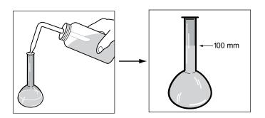
11. Weigh the 100 mL-soil/water mixture in the flask (without the stopper/cap). Record the mass of the mixture on the *Soil Particle Density Data Sheet*.
