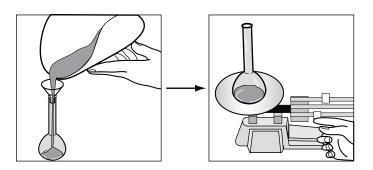
5. Measure the mass of the flask containing the soil (without the stopper/cap). Record the mass on the *Soil Particle Density Data Sheet*.
