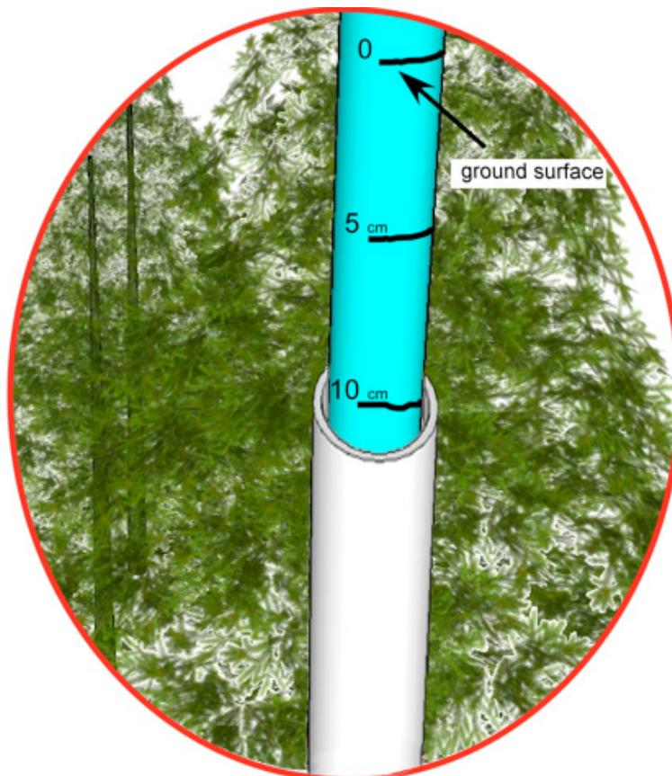
Figure 4. Another view of the Frost Tube showing inner outer tubes
