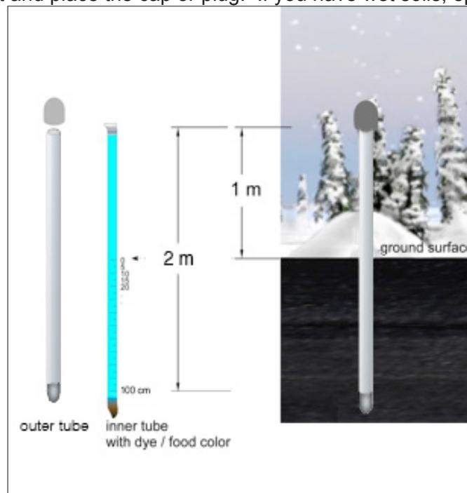
Figure 2. Frost Tube assembly showing liquid-filled inner tube (both ends sealed) and outer tube as well as the assembled frost tube placed in the ground.
