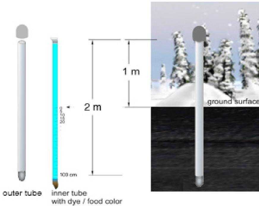
Figure 3. Components of a Frost Tube
