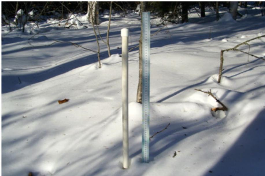
Figure 4. Assembled frost tube on left with a meter stick on the right
