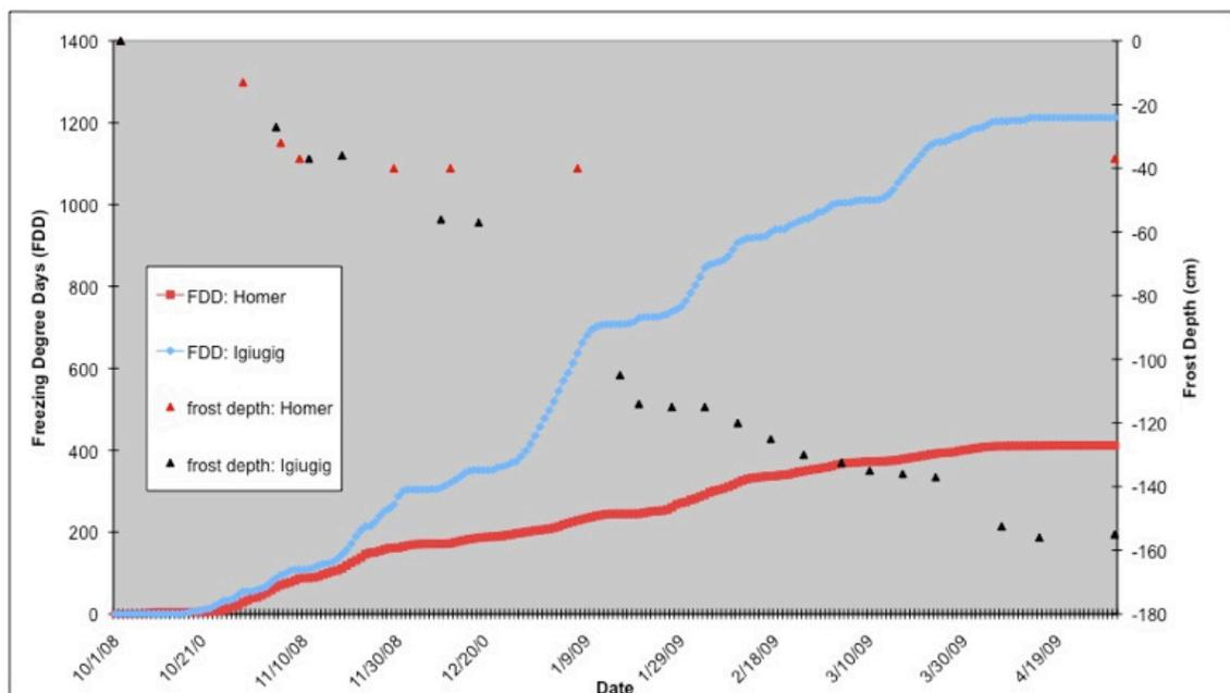
Figure 7. Freezing degree days and frost depths at Homer and Igiugig, Alaska
