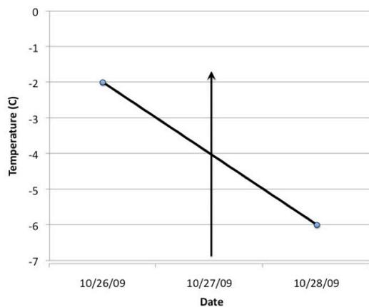
Figure 6. Estimate of missing datum for surface temperature on 27 October, 2008, at Homer.
