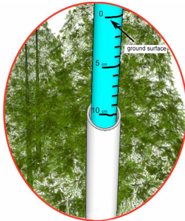
Figure 3. Ground surface and 5 cm below-ground increments with 1 cm hash marks on inner tube
