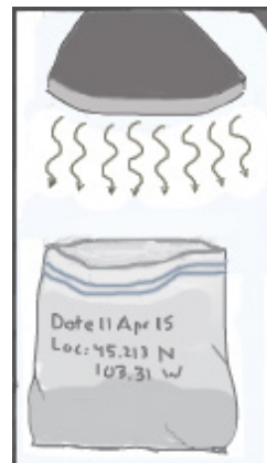
Figure 8, drying soil under a heating lamp
