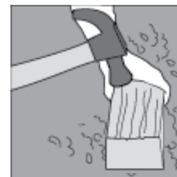
Figure 6, gently tap sample can with wood block and hammer
