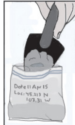
Figure 3, placing soil in zip lock bag
