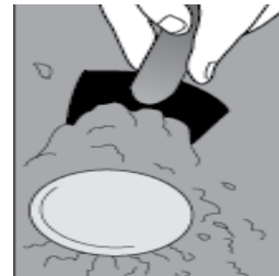
Figure 5, use trowel to dig up sample can
