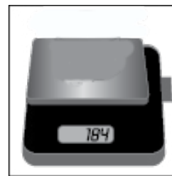
Figure 7, determine wet mass of soil
