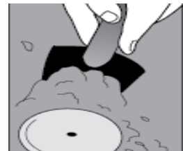
Figure 5. Use the trowel to dig up sample can.
