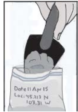
Figure 3. Place the soil in a sealable plastic bag.
