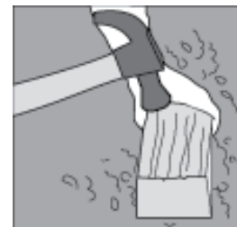
Figure 6. Gently tap the sample can with a wood block and hammer.
