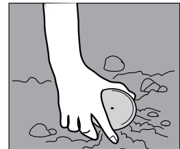
Figure 4. Push the sample can into the soil.
