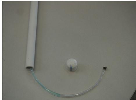
Figure 1b. Assembled Frost Tube
