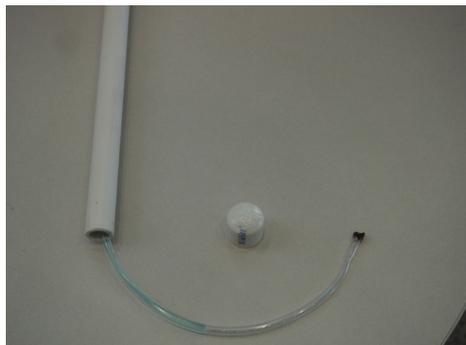
Figure 1b. Assembled Frost Tube
