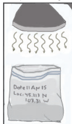
Figure 2, drying soil under heating lamp
