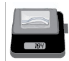
Figure 1, determine wet mass of soil sample and bag
