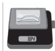
Figure 1, determine wet mass of soil sample and bag
