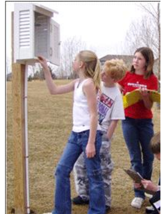
Installed Instrument Shelter
