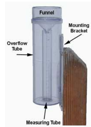
Installed Rain Gauge
