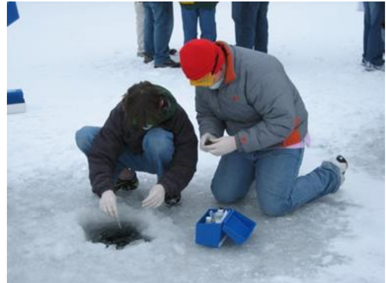
Students measure nitrate, pH and DO through ice covering the Volga River.
