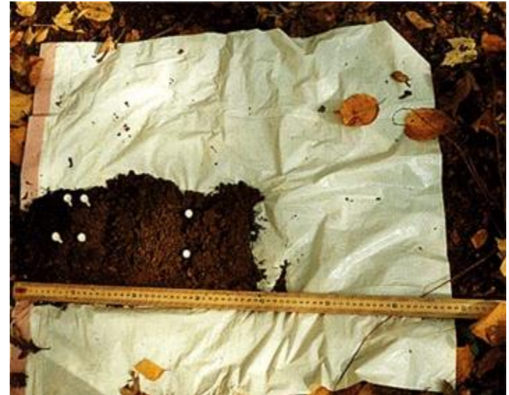
Augered soil profile with golf tees showing the horizons. Used with permission from Mid Valley Secondary Center, Throop, PA USA
