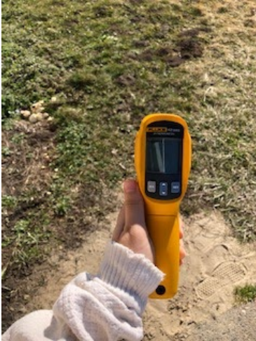
Figures 5-6: The infrared thermometer in figure five was used to take surface temperatures in nine locations around the tree. In figure six the PASCO wireless weather device was used to collect air temperature from under the tree for a consecutive ten minutes.
