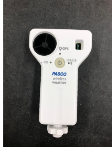
Figures 5-6: The infrared thermometer in figure five was used to take surface temperatures in nine locations around the tree. In figure six the PASCO wireless weather device was used to collect air temperature from under the tree for a consecutive ten minutes.
