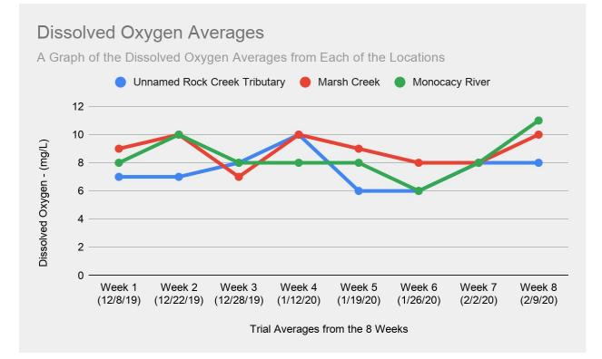
Graph 1: This graph shows the comparison of dissolved oxygen (mg/L) at the 3 testing sites. It is shown that the DO levels fluctuated from week to week. The most consistent average was from the three week testing (four week span), in the Monocacy River. Marsh Creek seemed to have stayed in the high road except for "Week 3." The DO stayed high, which is what is expected to see.
