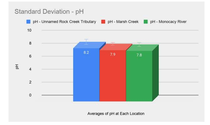
Graph 9: This shows the overall averages, from the raw data, of pH at each location. Standard deviation is a quantity calculated to indicate the extent of deviation for a group as a whole. The error bars show the variance of the row. The error bars show very little variance of the data. The levels of pH were a little higher than that which would have been thought. The recommended levels for pH were 6.5 to 8.
