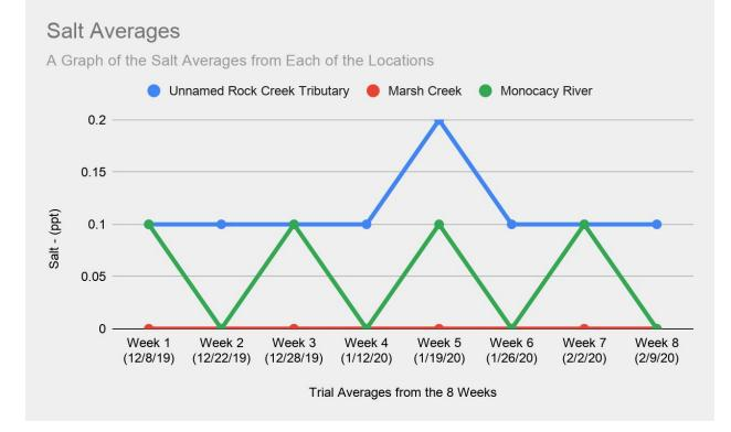
Graph 2: This graph shows the comparison of salt (ppt) at the 3 testing sites. The Salt stayed consistent and generally did not go above the 0.1 ppt line (except for the one week in the Unnamed Rock Creek Tributary), which is good.
