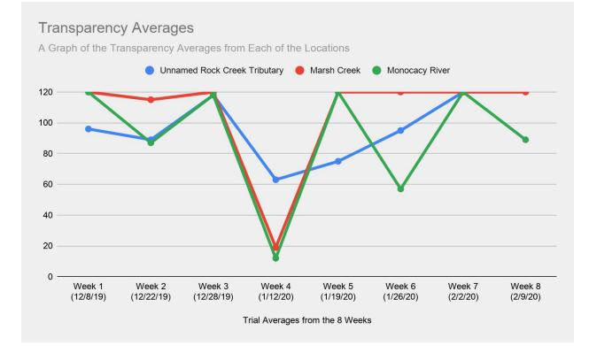
Graph 6: This graph shows the comparison of transparency (cm) at the 3 testing sites. The transparency shows that there is not a lot of sediment runoff going downstream (except for Week 4, which had a massive storm go through the area).
