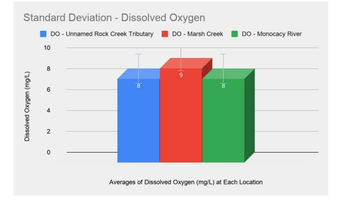
Graph 7: This shows the overall averages, from the raw data, of dissolved oxygen (mg/L) at each location. Standard deviation is a quantity calculated to indicate the extent of deviation for a group as a whole. The error bars show the variance of the row. The error bars show a medium amount of variance. This does fall within the accepted values, because it falls within the accepted values of 7mg/L and 10mg/L, which were the values of the raw data.
