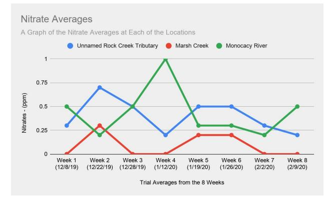
Graph 4: This graph shows the comparison of nitrates (ppm) at the 3 testing sites. The nitrates negatively and positively affect the water quality and the biodiversity. It is good that the nitrates do not exceed 1 ppm of the nitrates, showing that the streams are not picking up too many sediment pollutants.
