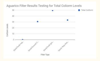
The following graph represents the effectiveness of the different filters tested for enterococcus, coliform, and e.coli levels. This supports that the sand/husk/regular charcoal filter performs the best in filtering out the contaminants.
